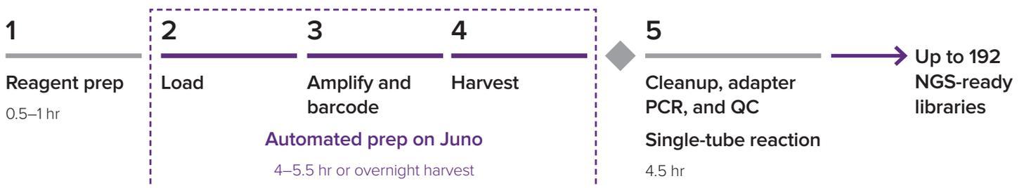
**Figure 1. Single run for the targeted DNA sequencing library preparation workflow on Juno.** Achieve greater operational efficiency and time savings by running a second integrated fluidic circuit (IFC) on Juno overnight and processing the amplified and barcoded product harvested from multiple Juno runs (Step 5) simultaneously.
